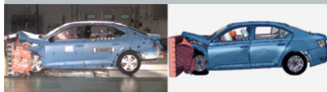
Physical test versus simulation of a frontal impact with ESI Virtual Performance Solution
