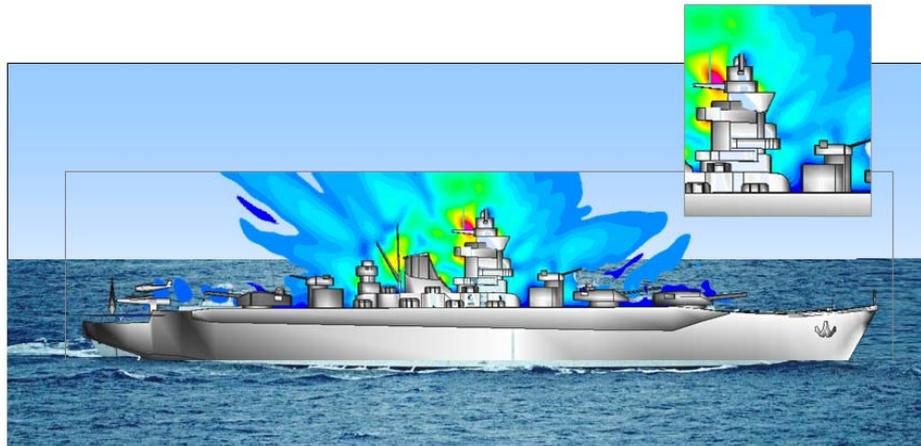
*Near Radiated Fields of an Antenna on a Navy Cruiser*
