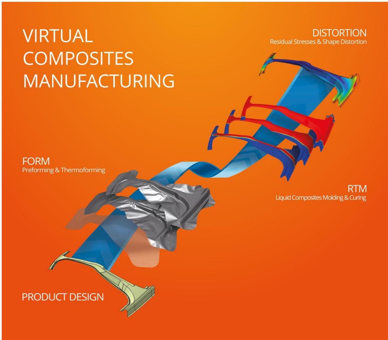
**Image:** Composites Simulation Solution 2015 enables the modeling and optimization of the different steps involved in manufacturing a structural composite part.
