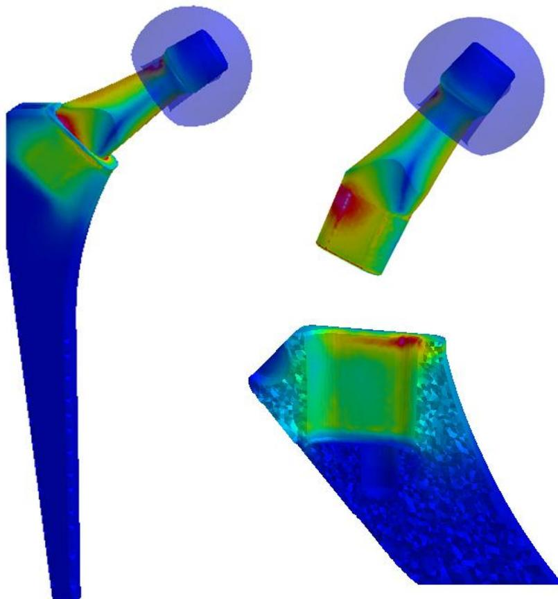
Image: Simulation results in Virtual Performance Solution: mechanical stresses for a given load case.
