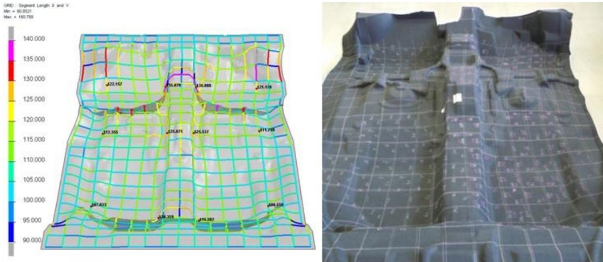
Image: Comparison between simulated grid with ESI PAM-COMPOSITES (left) and physical grid (right) on a synthetic automotive floor carpet
