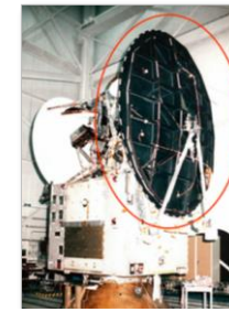
Qualification test for ribbed composite antennas
