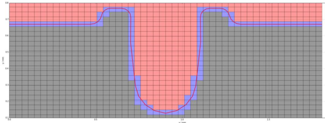
Figure 3: Micro-scale model generation with interface element identification.
