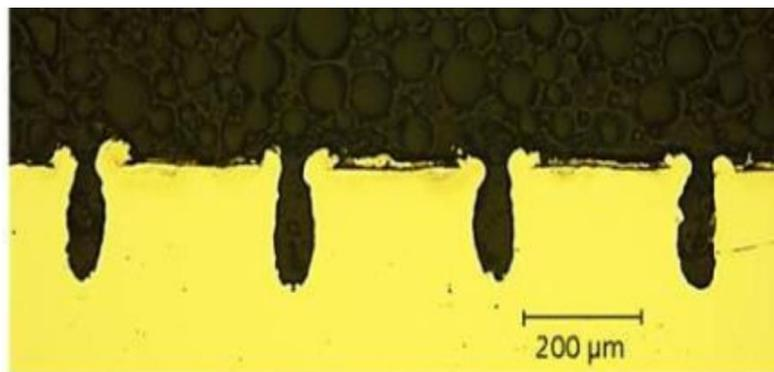
Figure 1: Micrograph of a laser structured composite-metal material interface.
