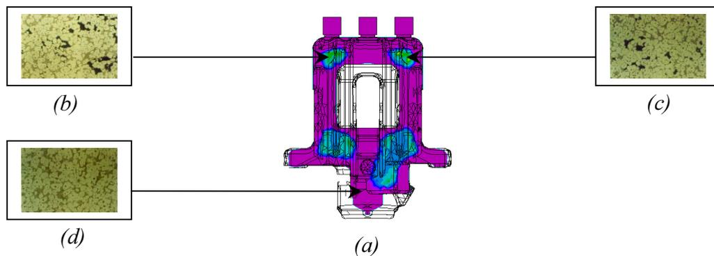
Figure 7: Contour plot of shrinkage porosity with micro structural results
