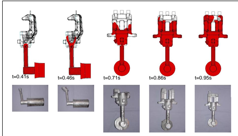
*Figure 3: Comparison of interrupted filling tests*
