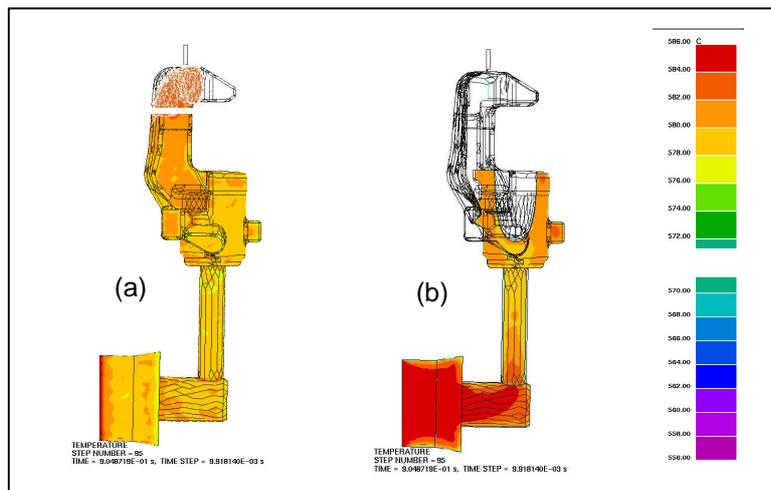
*Figure 4: Temperature contour plot showing premature solidification*
