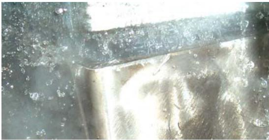
Figure 6. Water intrusion near the corner region showing that water intrudes mainly from the end face.
