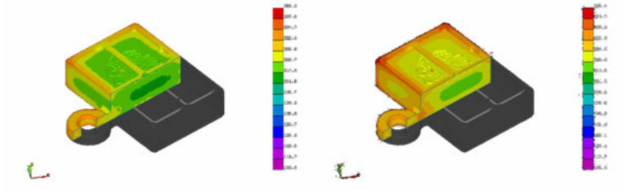
Figure 4: Tensile Strength plots display material property differences between a part that is shaken out after (left) versus before (right) solid state temperature is reached (ProCAST) (Pictures courtesy of Caterpillar, Inc., USA).
