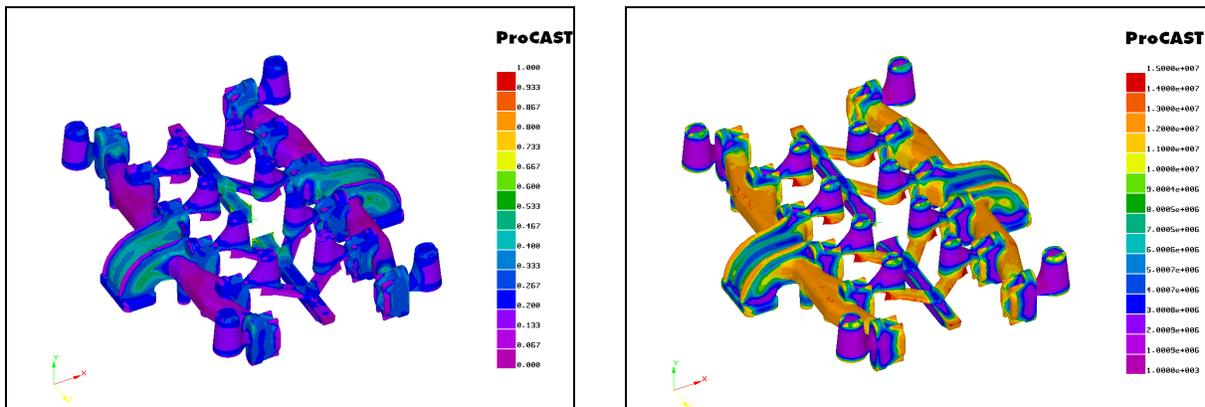
Figure 2: Fraction of ferrite (left), and nodule count (right), provide insight into the mechanical state of the as-cast part.
