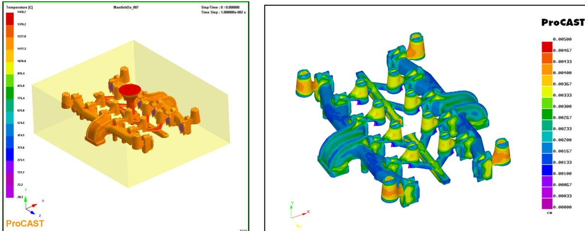
Figure 1: The chemical composition can be varied to identify the optimum mechanical properties configuration (SDAS results of ProCAST™ on the right and geometry with the gating, rising and sand mould on the left).
