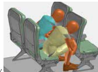
Simulation of an emergency landing for seat certification
