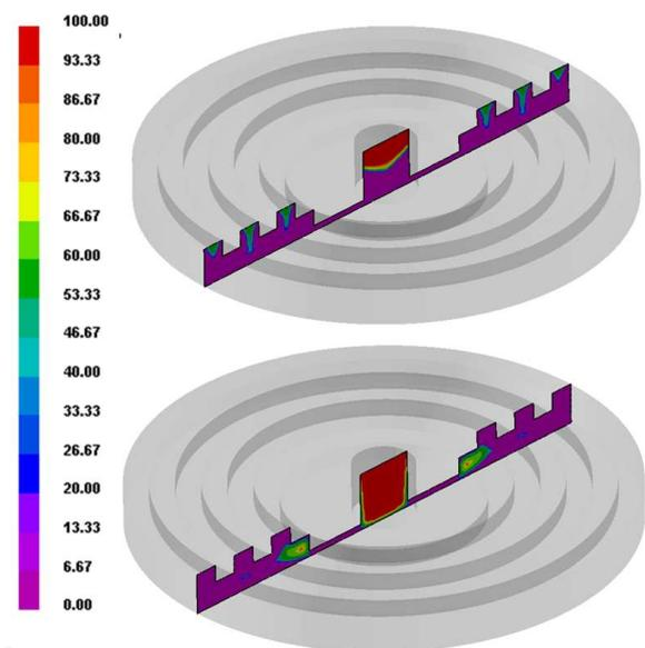
**Figure 2: Porosity formation under gravity influence (top) and centrifugal force (bottom). The scale is corresponding to the porosity level in percent**
