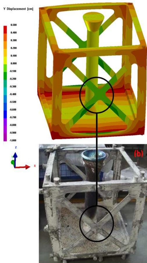
**Figure 4: Predicted and experimentally observed deformation of a cubic shaped frame.**
