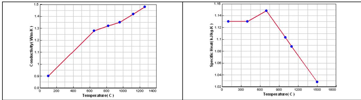
**Figure 6: Material Properties Ceramic Shell**
