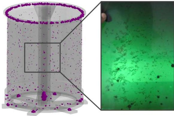
**Figure 10: Simulated and measured porosity distribution on the thin cylindrical section – first process design change**
