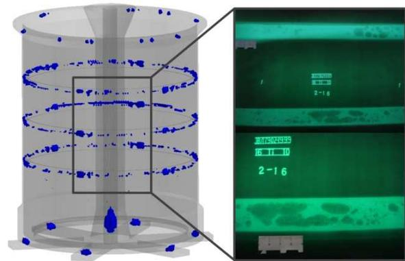
**Figure 11: Simulated and measured porosity distribution on the thin cylindrical section - second process design change with internal rings**
