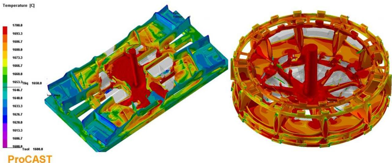
Figure 1: Casting modelling results of a doorframe component (left side) and an engine casing (right side) geometry
