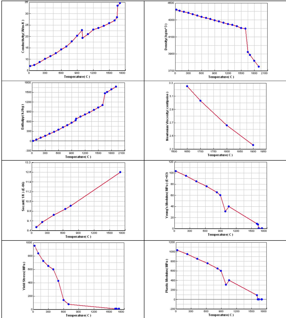
**Figure 5: Material properties Ti6Al4V**
