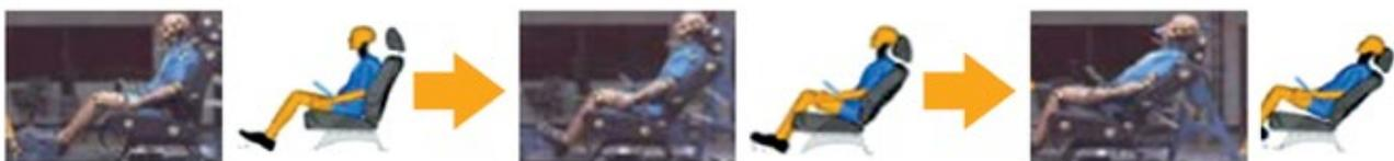
Virtual and real sled test with BioRID II.
