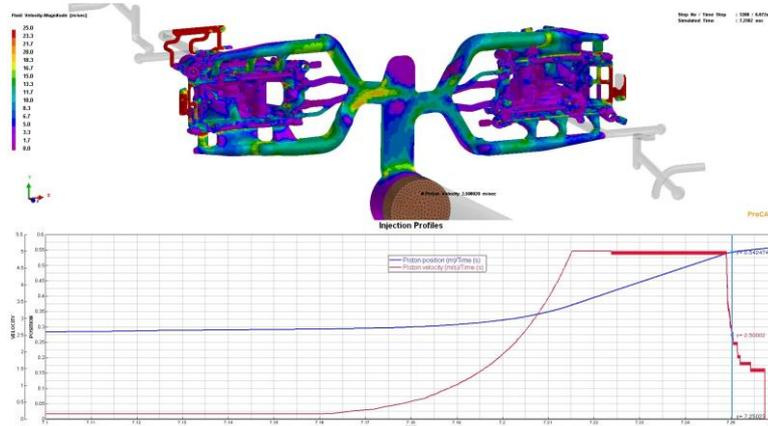
Image: ESI ProCAST simulation results using the new Real Time Piston Control feature.
