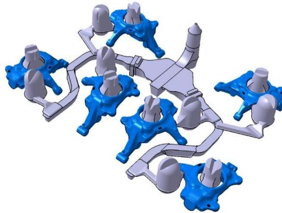
Fig1: 6-cavity mold layout derived from traditional approach
