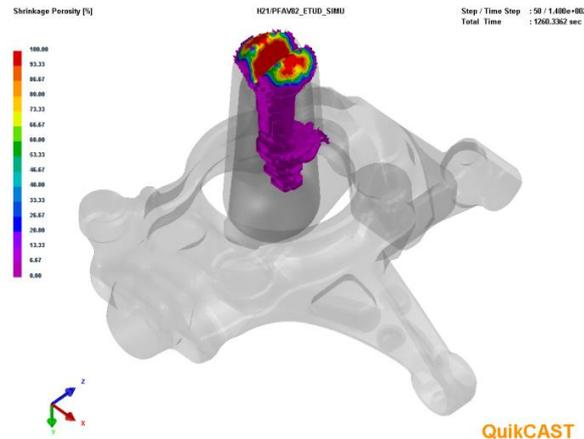
Fig6 : Design 5 shows the best feeder design , with no shrinkage in the casting part
